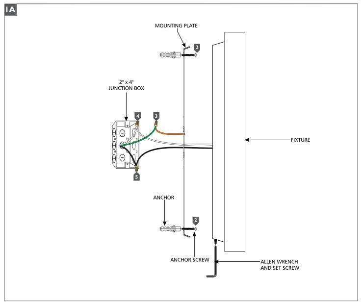
Separate the mounting plate from the fixture by loosening (do not remove) the set screw with the provided Allen wrench.
