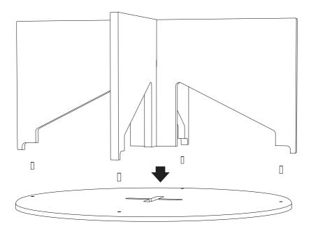
Place the top plate on the floor, add all four plugs in the table top and press legs inside. If needed rotate legs 90  $^{\circ}$  clockwise until perfect fit!
