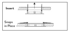
Holding spring clips against fixture, carefully insert the fixture into the hole. Continue to slide in the fixture, releasing spring clips, until clips snap into place. Ensure the fixture is flush against the ceiling and securely in place.
