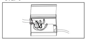
Make wiring connection inside the junction box using the EZ connectors (as shown above). Connect the 120V line wire from your house electrical to the black wire (black to black). Connect the neutral wire to the white wire (white to white). This fixture does not need to be grounded. Cap off the ground using a wire nut (1pc included).
