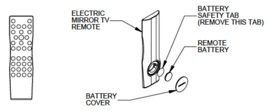
Power up the TV unit and test audio and video functionality. The LCD TV operates by remote control only. Take the batteries out of the remote. Remove the safety tab, place the batteries back inside and close. Turn TV on. Hit the source button to search for RF source. Hit the scan button to auto scan the TV to cable channel. Refer to the TV Operation Manual for instructions on how to operate the TV.
