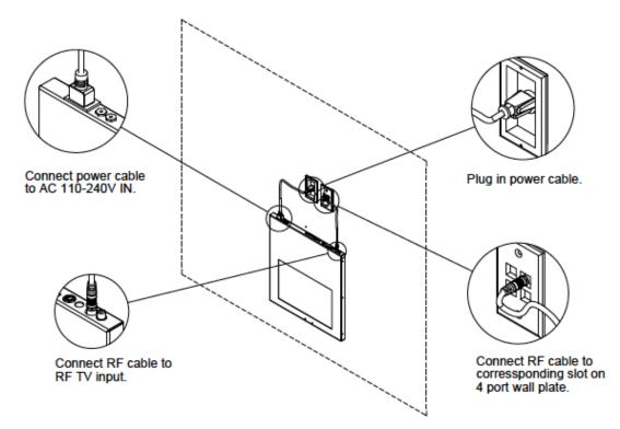
Connect Power and Video. Move the Mirror TV close to the final position and plug the power, video, and audio cables (from the integrated mini speakers) into their appropriate sources. An RF cable is provided. Before hanging the unit, ensure that cables have sufficient slack.
