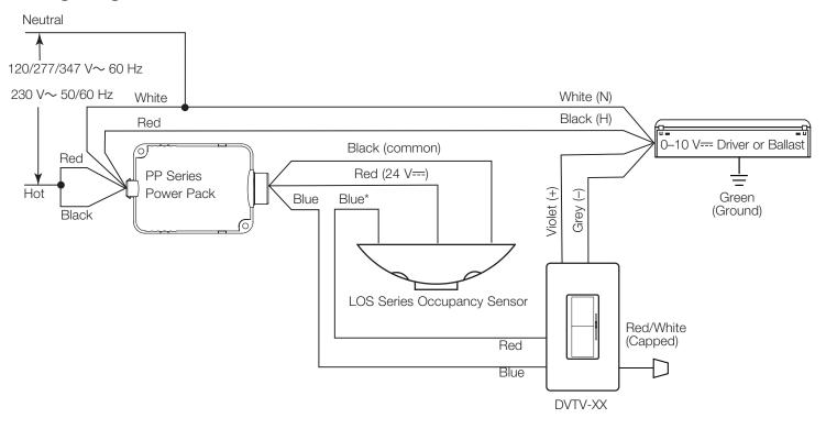
\* For LOS-CDT-500R-WH, LOS-CDT-1000R-WH, LOS-CDT-2000R-WH, and LOS-WDT-R-WH models: Use the gray wire instead of the blue wire to use the photo cell option. The photo cell option prevents the lights from turning on when there is sufficient natural light and is available only with these –R models. These models also contain a separate relay output (yellow/white, black/white, and blue/white wires) that is not needed for this installation.
