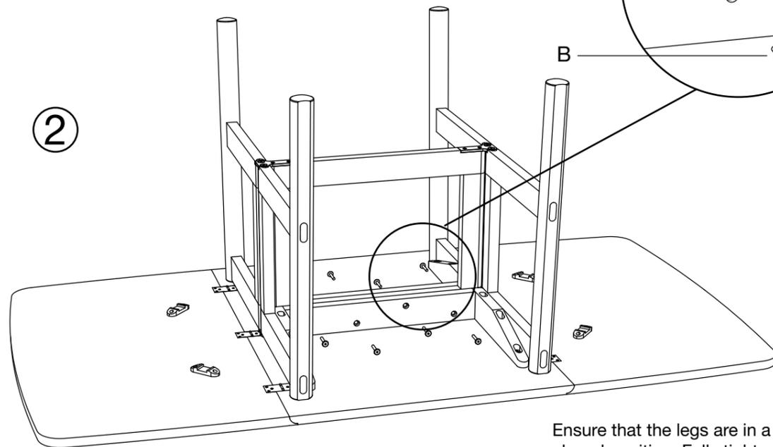
Ensure that the legs are in a closed position. Fully tighten A and B together using 2 x Allen key C.
