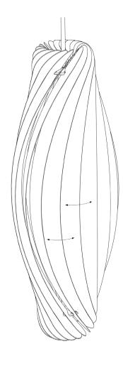
1) Remove all parts from the box and insert a lightbulb into the E14 socket
