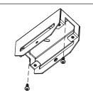
Pass sectioned flat cable in strain relief in canopy in direction of support box 3 and the other one in direction of support box 5. (Loosen captive screws for better passing of cable)
