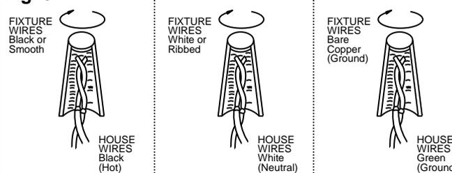
**IMPORTANT: FIXTURE SHOULD BE INSTALLED BY A QUALIFIED ELECTRICIAN TO ENSURE PROPER WIRING AND INSTALLATION.**
