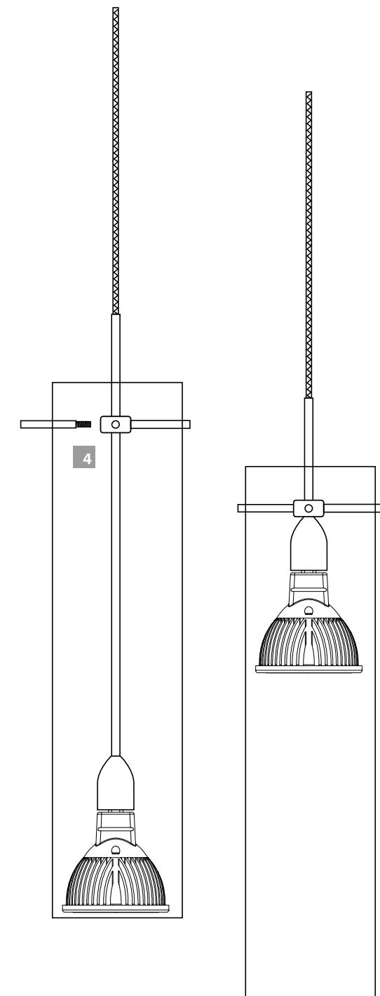
**4** Place the glass shade completely into the ring and tighten the three thumb screws to secure the glass shade in place.
