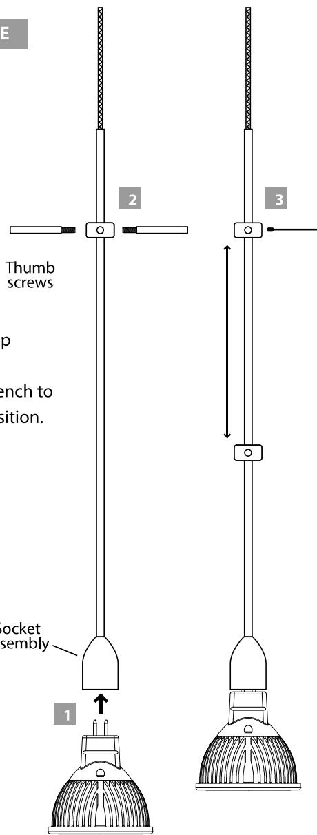
**2** Remove the three thumb screws.
