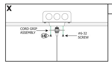
**18:** Mount the cord grip assembly to the 2" plaster ring using two #6-32 screws.
