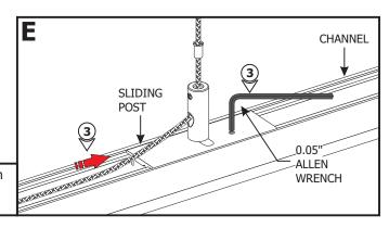
**3:** Carefully move the sliding post to the predetermined location on channel and tighten the #4-40 set screw on the sliding post bed with the 0.05" Allen wrench.
