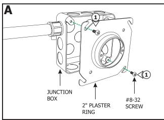
**NOTE:** Junction box must be mounted to allow clearance of 1/2" between the face of the junction box and the drywall surface.
