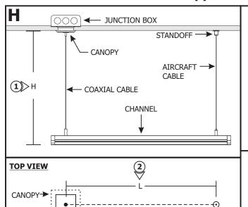
**NOTE:** Run the proper size wires between the 24VDC power supply to the electrical box. Refer to the instructions provided with the power supply for additional information.
