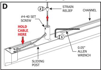
**WARNING:** To avoid damaging the coaxial cable electrical connection, make sure that the end of the coaxial cable coming out of the fixture is held with thumb before relocating sliding posts.
