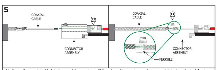
**11:** Insert the coaxial cable into the coaxial connector until the wires of the center conductor are visible through the M3 set screw hole.
