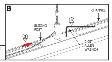
**3:** Carefully move the sliding post to the predetermined location on channel and tighten the #4-40 set screw on the sliding post bed with the 0.05" Allen wrench.
