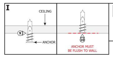
**NOTE:** Steps 9 and 10 are for drywall mounting. Omit these steps if mounting directly to a wood surface.
