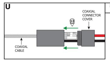
**13:** Replace the coaxial connector cover and tighten into place.
