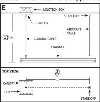
**NOTE:** Run the proper size wires between the 24VDC power supply to the electrical box. Refer to the instructions provided with the power supply for additional information.
