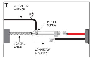
**12:** Use the provided 2mm Allen wrench to securely tighten the M4 set screw until it squeezes the wire ferrule tightly to the coaxial cable.
