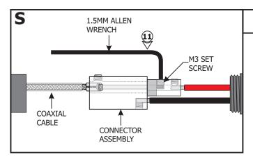
**11:** Use the provided 1.5mm Allen wrench to replace and securely tighten the M3 set screw.
