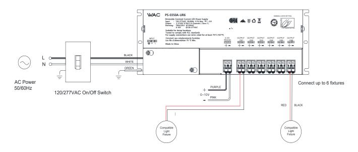
\*Note: Longer distance than 100ft between power supply to light fixture requires larger conductor wire than 18 AWG to lower voltage drop across the wire. Excessive voltage drop on conductor wires may lead to an inoperative of power supply.
