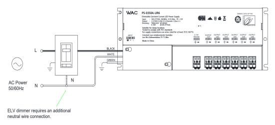
\*Note: No dimming curve adjustment function for Phase Cut dimming.
