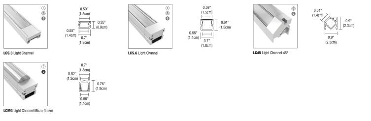
RECESSED LIGHT CHANNELS: Recommended applications\* (Recessed into drywall or wood)\*\* — Coves, pathways, toe-kicks, undercabinets, and shelves
