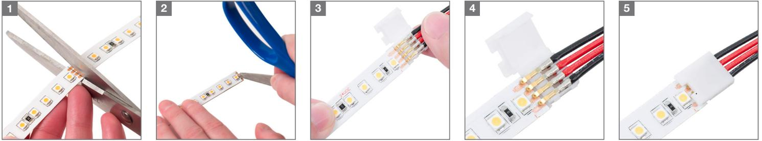
**Using the Snap & Light Solderless Connectors:** Cutting and reconnecting our LED Stomp Strip is easy. All you need is a pair of scissors or any sharp device that will allow you to make a clean cut.
