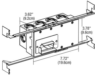
**PURE SMART 4 GANG JUNCTION BOX WITH MOUNTING PLATE (INCLUDED WITH TL1.6A COMPLETE FIXTURE ORDERING CODE)**
