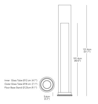
\* Components drawn in relative scale. Refer to CAD files for accurate drawings.
