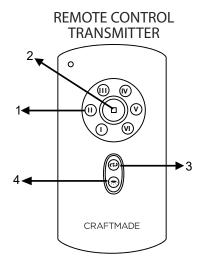
**1**--Fan **SPEED** buttons: Use to control fan speeds 1-6
