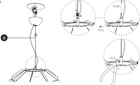
3. Adjust the height of your lamp by raising or lowering the stainless steel adjustment cable (G) and cut off the excess.
