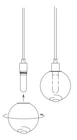
Figure 5. Install glass spheres by threading onto brass sockets
