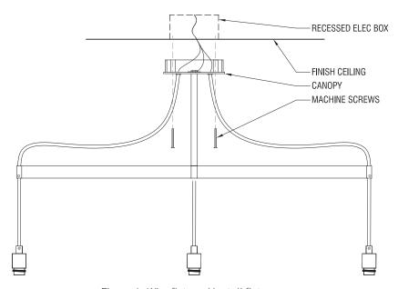
Figure 4. Wire fixture / Install fixture
