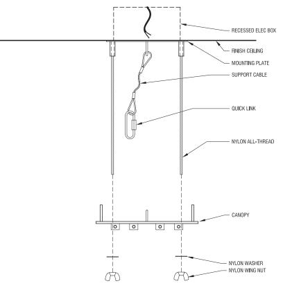
Figure 3. Install nylon all-thread rods into mounting plate and slide canopy up over rods
