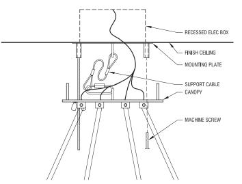
Figure 7. Fasten canopy to mounting plate
