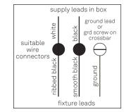
Figure 6. Wiring Diagram
