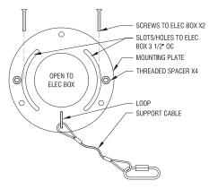
Figure 2. Install mounting plate
