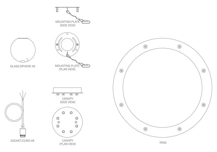
Figure 1. Parts of the Light Fixture
