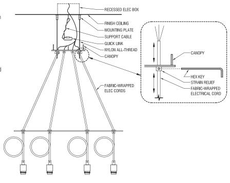
Figure 5. Leveling the fixtue
