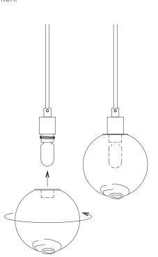
Figure 8. Install glass spheres by threading onto brass sockets
