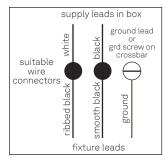
Figure 2. Wiring Diagram
