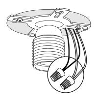
NOTE! NEATLY TUCK WIRES AND CONNECTORS UP INTO THE JUNCTION BOX.
