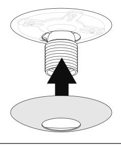
**4** Secure SHADE to SOCKET using the CHECK RING. Install the bulb.
