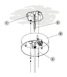
The canopy is made up of a back plate with the electrical connections on it and a front cover. Feed the electrical wires (A) from the mains through the electrical back plate (B), fix back plate to the junction box (1) with the most adequate screws (C) (not supplied) and prepare to wire up.
