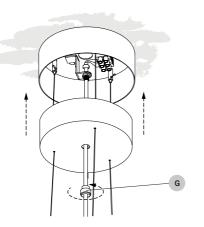
Once all your wiring is complete raise the canopy and screw on the canopy support nut (G) that holds the cover in place.
