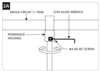
To lock the fixture head in a permanent horizontal position, tighten the #4-40 set screw on the PowerJack housing with the provided 0.05 Allen wrench.
