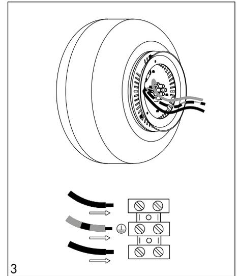
Connect to electricity using the terminal block.
