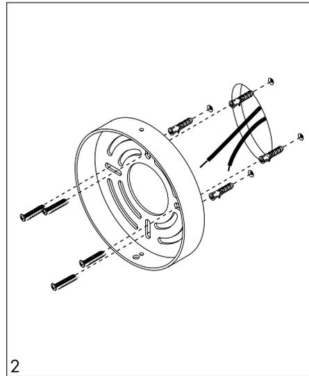
Fix the mounting plate to the wall with dowels and screws.
