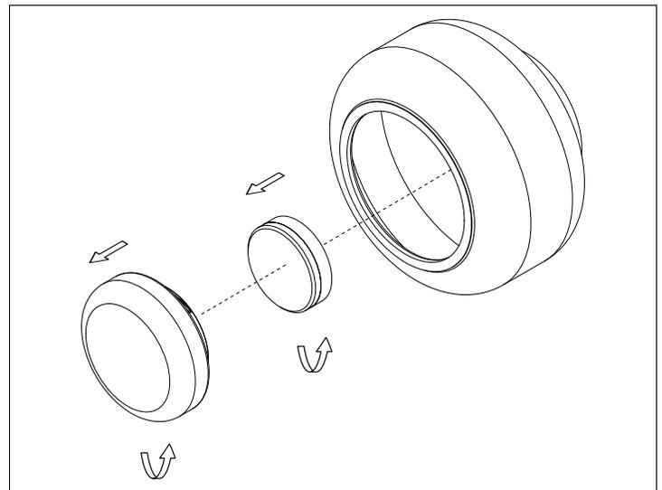
**Bulb change:** Spin off the inside opal glass, the spin off the Gx53 Bulb.
