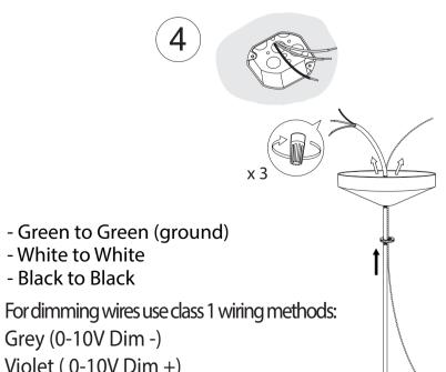
For dimming wires use class 1 wiring methods: Grey (0-10V Dim -)
