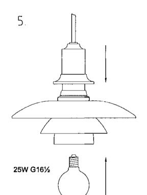
Fine adjustment of the incandescant lamp.
