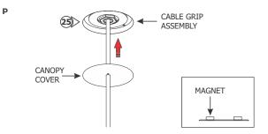
26 If necessary, use fingers to push on the perimeter of the canopy cover until it slightly rocks and lift the cover to remove it from the assembly.
