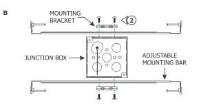
**NOTE** Adjustable mounting bars mount to studs that are spaced 14.5" to 25" apart.
