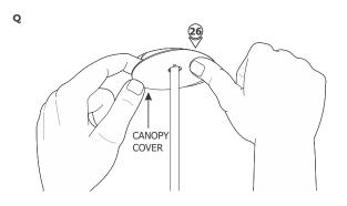
**NOTE** If using metal tools to apply plaster, be careful not to remove the magnetic canopy cover while plastering.
