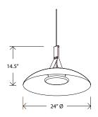
Dimensions: 24" Ø, 14.5" Product weight: 7 lb Light Source: integrated LED Light output: 2625 Lumens (source)
