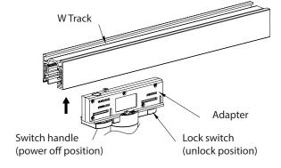
2. Make sure the convexity on the adaptor box is at the same side with the slot on the track (Fig 2). Fit the adaptor box into the track. Ensure the convexity on the adaptor box is at the same side with the slot on the track.
