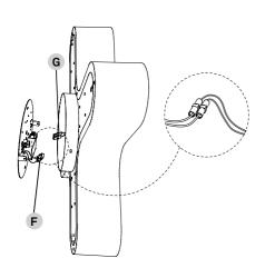
Take the connector from the Driver (F) and connect it to the shade connector (G).
