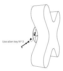
Return the shade to its position. Put the holding screws back into place.
