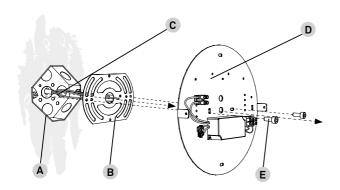
Feed the electrical wires (C) in through the back plate (B) and wall light backering plate (D).
