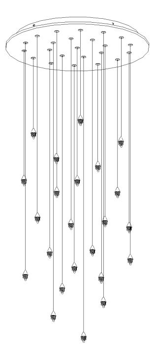
**5** If your chandelier is not pre-staggered (most standard length fixtures are not), stagger it to the desired design. You are able to make adjustments to the wire lengths if necessary using the provided metal grippers on the canopy. SEE BELOW.
