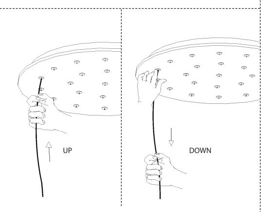
**6** To adjust wire lengths: NEVER TUG ON WIRES! The fixture comes assembled at the maximum length. Lengthening a wire can only be done once it has been shortened. Never try to lengthen wires past the maximum length.
