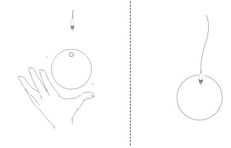
7 Once the fixture is mounted and wires have been adjusted, attach your glass pendants. Ensure sockets are cool to the touch before proceeding.
