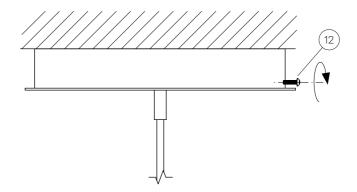
Screw the diffuser 3 into the thread in the mounting 2.
