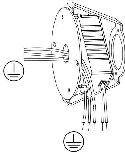
**D** Secure the electrical bracket to the outlet box with two screws (not provided).
