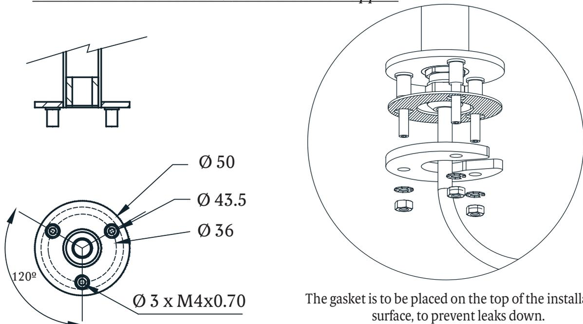
The gasket is to be placed on the top of the installation surface, to prevent leaks down.
