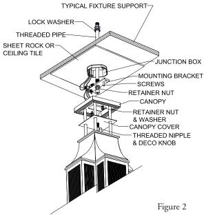
Step 2 Locate outlet box and with the power turned off at the circuit attach the mounting bracket to the outlet box. Include a structural member such as a steel angle bracket or stud that is secured into the ceiling and meets local building codes. Route the steel pipe up and through the center of the outlet box and through the additional support member. The threaded pipe can be cut to length. Use additional hardware to fasten the pipe and mounting bracket securely to the ceiling. (See Figure 2)
