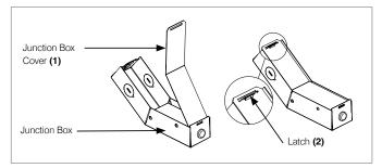
Insert the 120/277V supply lead through the knockout in the junction box. Make the electrical connections according to the wire colors: White/White, Black/Black, Green/Green and 0-10V dimmers if needed (see wiring diagram).
