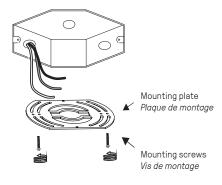
Connect supply wires to wires on fixture with wire nuts or push wires into quick connector. Connect white to white, black to black, and copper wire to copper wire as grounding connection.
