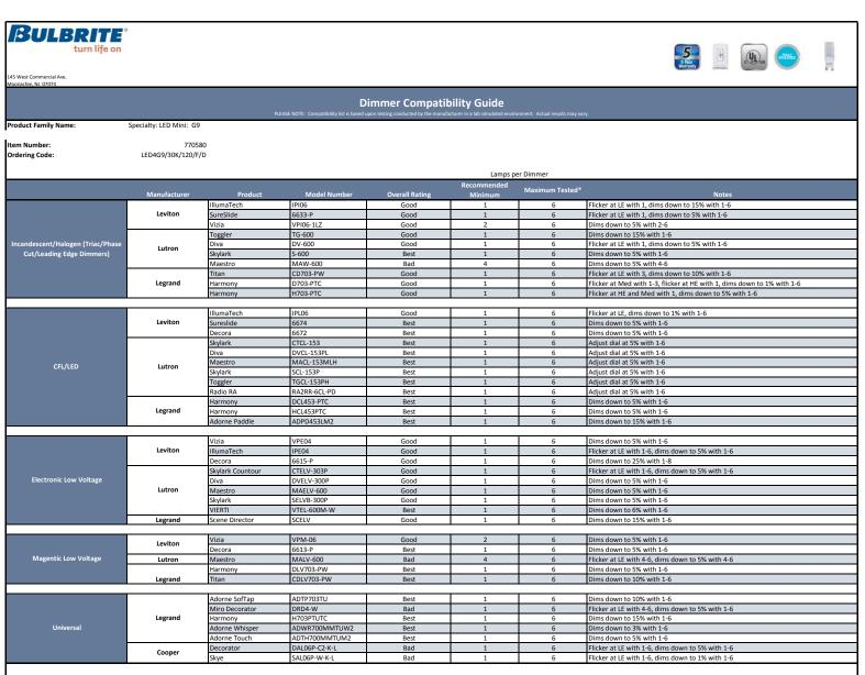
Maximum Tested (Lamps per Dimmer) - Additional lamps may work with your dimmer system. For maximum capacity please consult dimmer manufacturer
