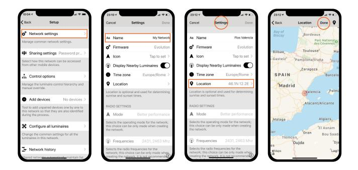
The network *Mode* has two options: **Balanced** and **Better performance**. Most types of network should use **Balanced** mode. Although networks with a large number of devices which are very close to each other (i.e. over 100), **Better performance** mode can be selected.
