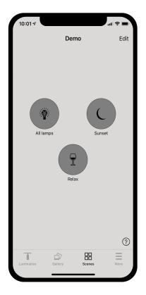
Select *Edit* and + then enter a name for the scene and select *Add a scene*. Select and adjust the luminaires for this scene. With + you can add all luminaires and with - you can remove all luminaires from the scene. You can adjust the luminaires separately or if you want to have same dim level or colour for all you can use *Luminaires in scene* control to adjust all luminaires in the scene.
