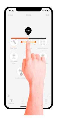
Tip: use the basic gestures on the All luminaires icon to control all of your lamps simultaneously or Nearby luminaires icon to control luminaires that are close to you.
