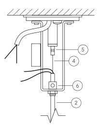
The steel cable is secured by inserting into the reutlinger.
