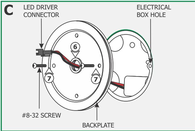
**6:** Feed the LED driver connector into the back of the gasket and backplate.
