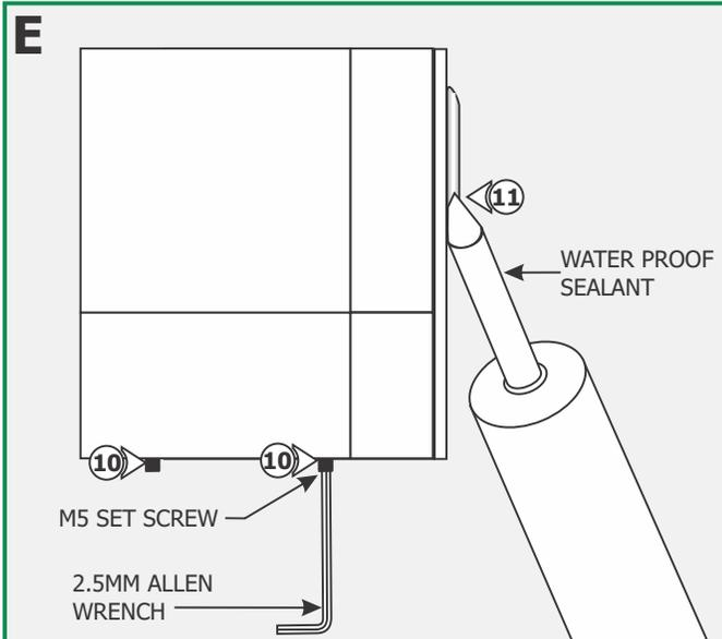
**10:** Place the fixture completely onto the backplate. Tighten the two M5 set screws on the bottom of the fixture with the 2.5mm Allen wrench.
