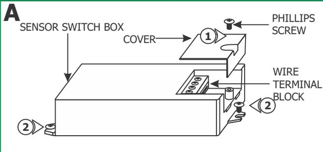
**1:** Loosen the Phillips screws on top of the sensor switch box to remove the cover exposing the terminal blocks.
