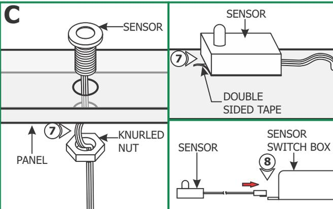
**6:** Install sensor within 3 feet of the sensor switch.
