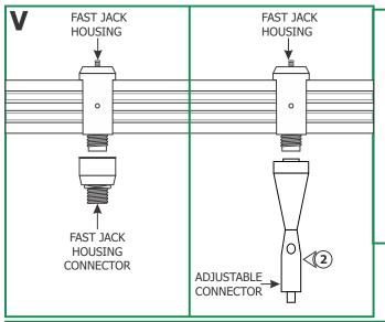
**NOTE:** To install the aircraft cable side of the fixture onto the ceiling, follow steps 3 through 11 and 13 in the "Install Cirrus Float to Single or Multi Port Fast Jack Canopies" starting on page 4.
