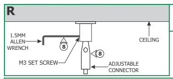
8: Insert the adjustable connector completely into the threaded post and tighten the M3 set screw with the 1.5mm Allen wrench.
