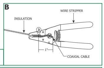
**3:** Use the #12 gauge hole of the AWG wire strippers to strip 1" of the insulation cover from the end so that the bare coaxial cable is exposed.
