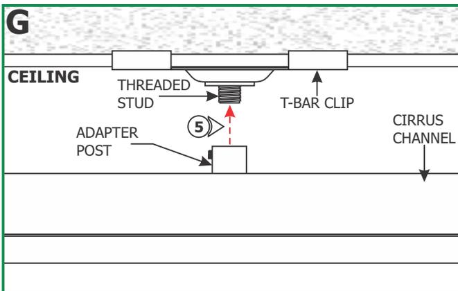
**5:** If necessary, slide the T-bar clips to align with the T-bar clip adapters. Align and insert the T-bar clips adapter posts into the threaded studs.
