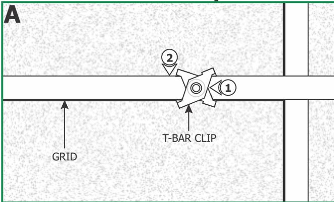
**1:** Open the T-Bar clip arms to fit over the grid.
