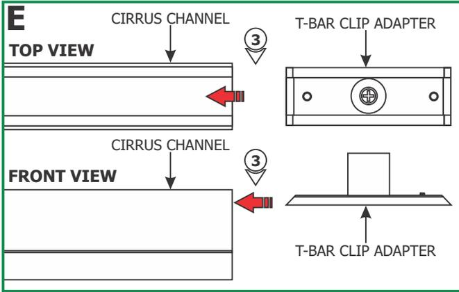
**3:** Slide the T-Bar clip adapter(s) into the Cirrus channel.
