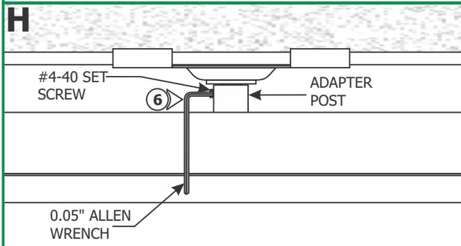
**7:** Replace the end cap to the end of the channel and tighten two #4-40 set screws with a 0.05" Allen wrench.
