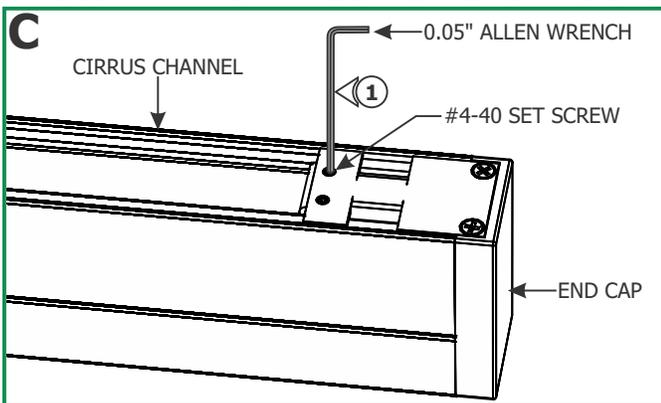
**1:** Loosen the two #4-40 set screws (**DO NOT REMOVE**) on the end cap at the non-power side of the Cirrus channel using a 0.05" Allen wrench.
