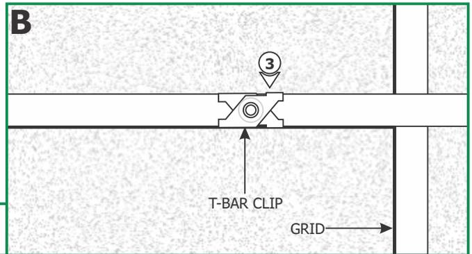
**3:** Place the T-Bar clip onto the grid and squeeze the arms together to secure it in place.
