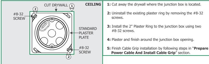
**NOTE:** Junction box must be mounted to allow clearance of 1/2" between the face of the junction box and the drywall surface.
