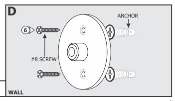
**6:** Mount each base to the anchors with two provided #8 screws.
