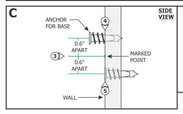
**NOTE:** The base holes should be in a vertical position at 90° angle to the direction of the fixture.
