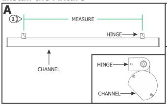
2: The hinge containing power wires should be aligned with the center of the junction box. Starting from the center of the junction box, mark all measured point(s) onto the wall ensuring the marked points are leveled horizontally with the center of the junction box.
