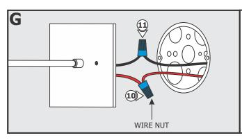
**NOTE:** The 24VDC power wires must be present to the junction box. Refer to the installation instructions provided with power supply.
