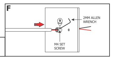
**9:** Feed the power wires coming out of the stem through the square canopy. Slide the canopy bushing completely onto the stem and secure it in place by tightening the M4 set screw with the provided 2mm Allen wrench.
