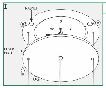
**6:** Slide the cover plate up against the mounting plate, the magnets will hold the cover plate in place.
