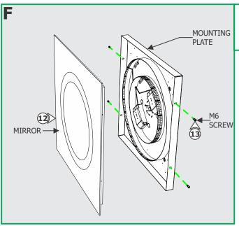
**12:** Carefully place the mirror onto the mounting plate.
